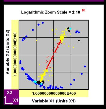
In this second example, the particles converge down through 16 orders of magnitude in spatial scale to the solution (having the 15 decimal place precision of Excel).
