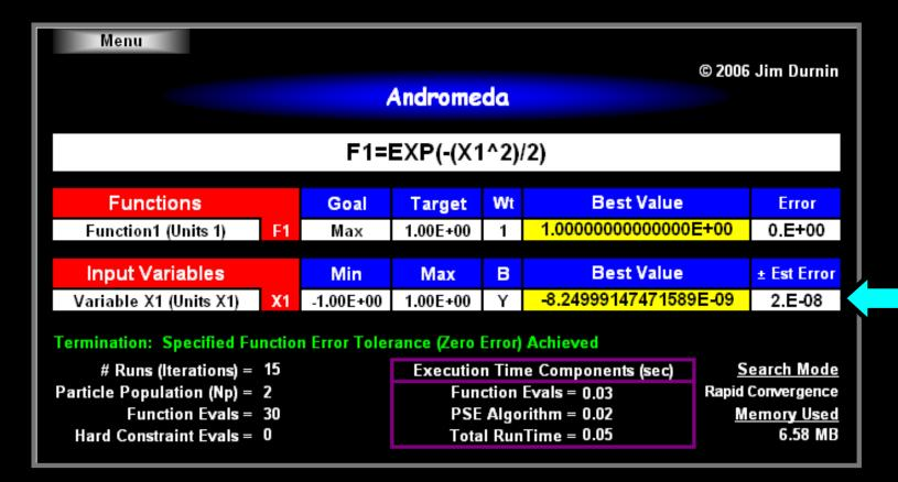
A novel aspect of the PSE algorithm is that the particle density provides an accurate estimate of the Error in the solution values at every step of the particle evolution.
