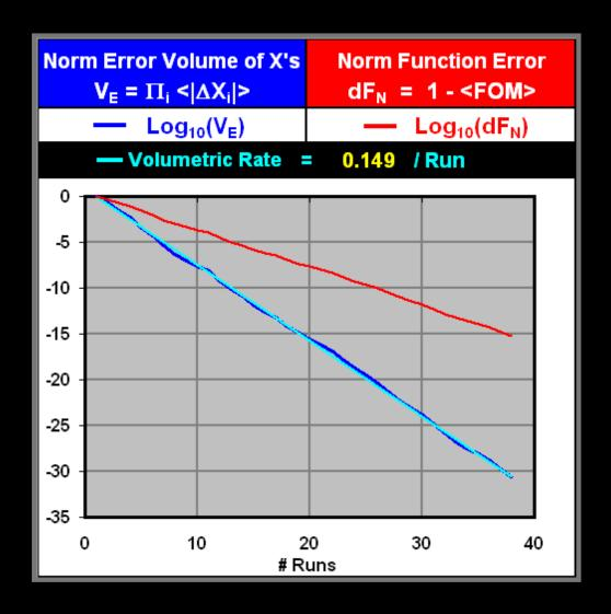
The convergence plot is provided as a tool for those who wish to study the convergence properties of the PSE algorithm. It shows the reduction in both the Error Volume of the X's and the Function Error versus the number of runs (iterations).
