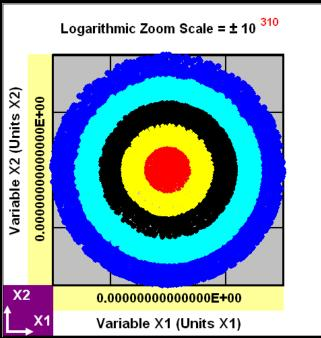
In this first example, the particles converge down through 310 orders of magnitude in spatial scale to the solution (representing the machine value of Zero in Excel).
