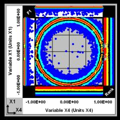
An example of matrix contour plotting the particle positions after only 10 iterations of the PSE algorithm to reveal the detailed structure of the solutions to the 4 dimensional optimization problem shown below.
